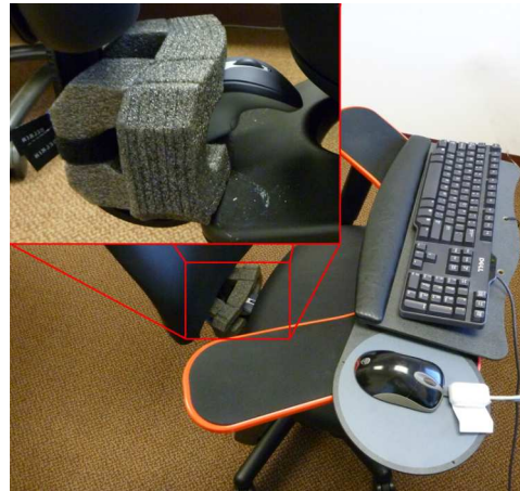
Figure 3 ChairMouse with keyboard and mouse attached to armrests. A GyroMouse attached under the seat captures chair
